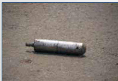
Damaged Source Outside Shield
