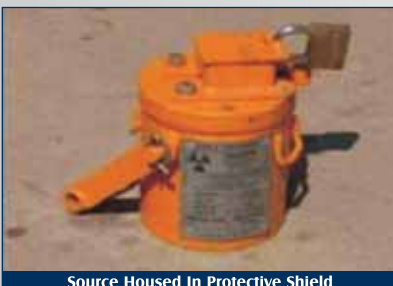
Source Housed In Protective Shield
